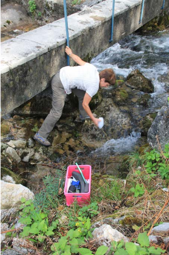
Measurement of physical parameters and sampling of water for chemical analysis at the Hubelj spring.
