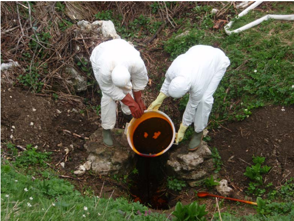
A fluorescent tracer uranine was injected in a karst fissure on April 24, 2014.
