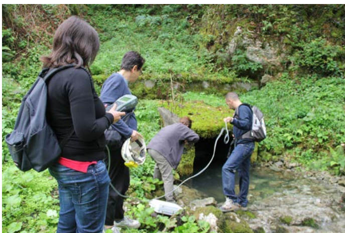
Measurement of physical parameters and sampling of water for chemical analysis at the Kajža spring.
