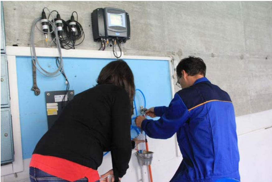
Measurement of physical parameters and sampling of water for chemical analysis at the Mrzlek pumping station.
