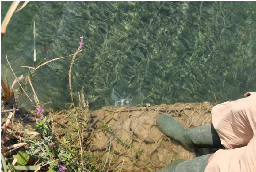
Installation of divers for measurement of water level, electrical conductivity, and temperature at the Soča River.
