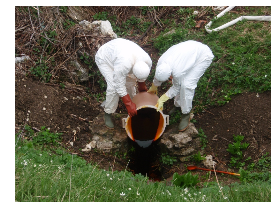
Injection of 6 kg of uranine into a fissure on the karst surface at the Malo polje area.
