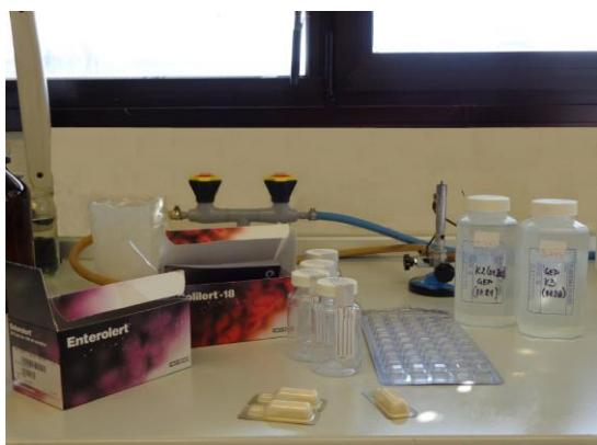
Slika 2: Reagent Colilert in Enterolert, stekleničke, Quanti-Tray in vzorca vode
